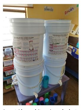
can be easily adapted to any container. This ceramic cartridge and its universal adapter "Aguadapt" are manufactured by Caminos de Agua, an NGO based in Guanajuato, Mexico, in collaboration with Concern's Appropriate Technology team.
